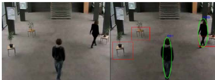
Figure 7: Input and output picture of the OpenCV Surveillance Facility library for motion tracking. In the given example, objects of interest are represented by plants. The library detects the users present in the scene and gives 2d position estimates over time.
