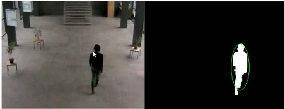
Figure 8: Example for a foreground / background detection. On the left-hand side, the raw image is given, while the result of the foreground / background detection is given on the right-hand side.
