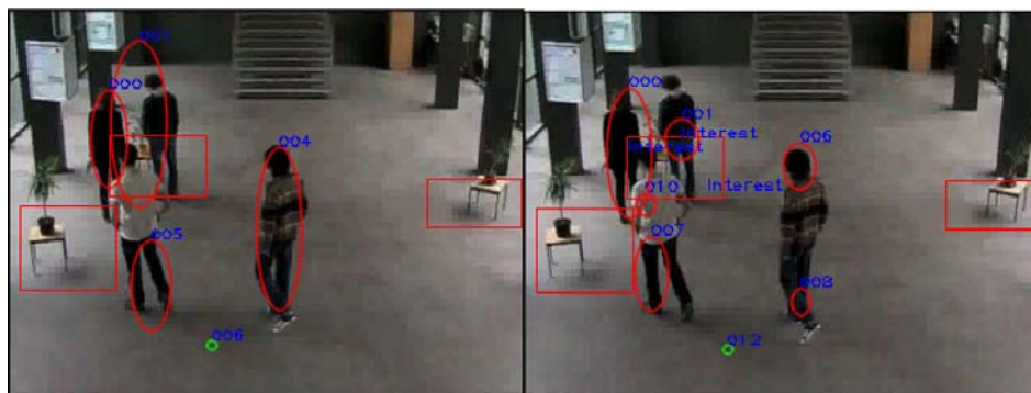
Figure 9: More complex scene processed by the blob tracking module using two different algorithms, i.e., the CCMSPF method (image on left-hand side) and the MSPF method (image on right-hand side). The CCMSPF method appears to deliver more useful results for the tracking of detected users.
