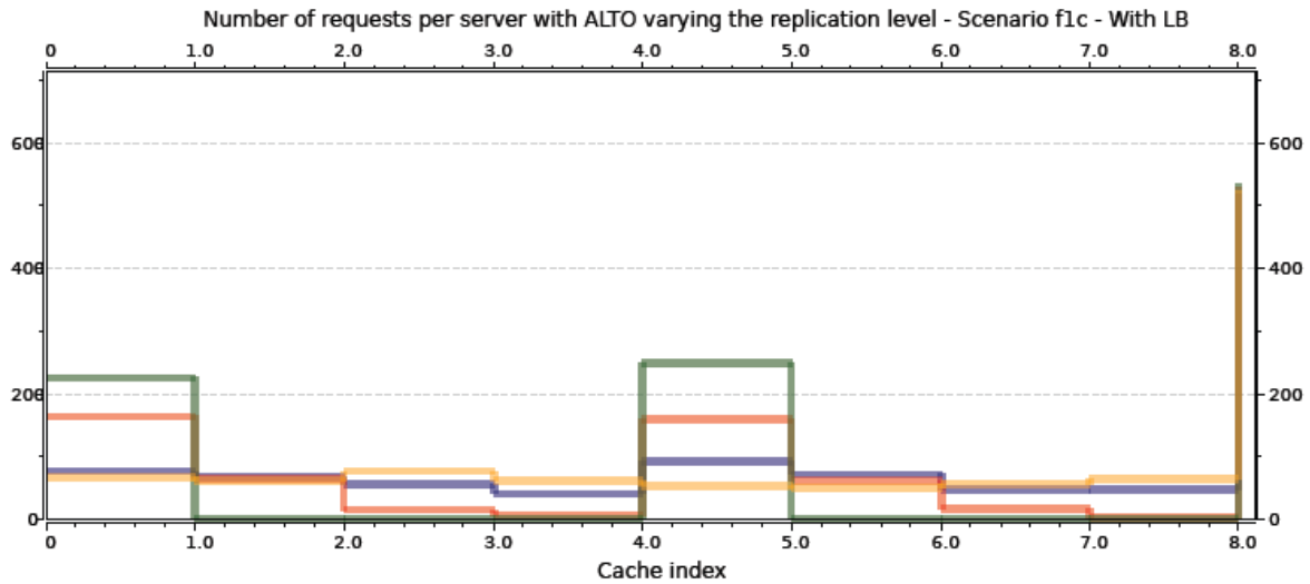
Figure 31: Number of requests per server with ALTO cache selection and with load balancing for different values of replication level
